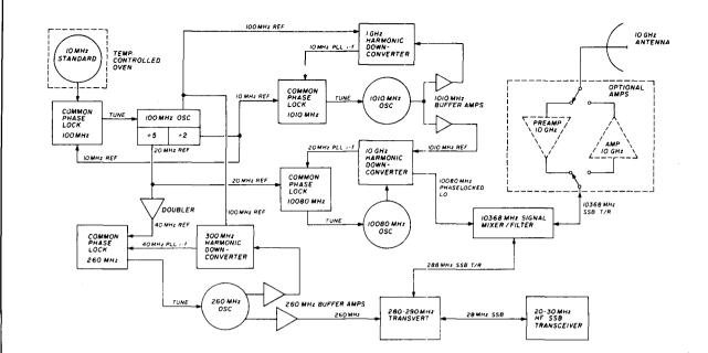
fig. 3. A precise 10,368 MHz SSB station can be made from only 5 oscillators and 4 nearly identical phaselock circuits. The PLL downconverters are similar in topology and easy to construct.
